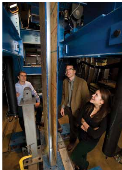
Ben Schafer (center), with grad students Luiz Vieira and Kara Peterman, uses the Big Blue Baby to study how seismic forces affect mid-rise cold-formed-steel buildings.
